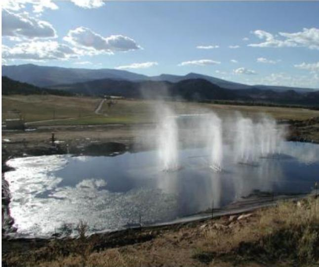
Due to the expense of proper disposal of fracking fluids, many drilling companies use misters to spray wastewater into the air so as to speed evaporation,<sup>30</sup> thus reducing the volume of waste fluids. This has the effect of transferring toxic substances from the water to the air, where they may cause harm to health via inhalation.
